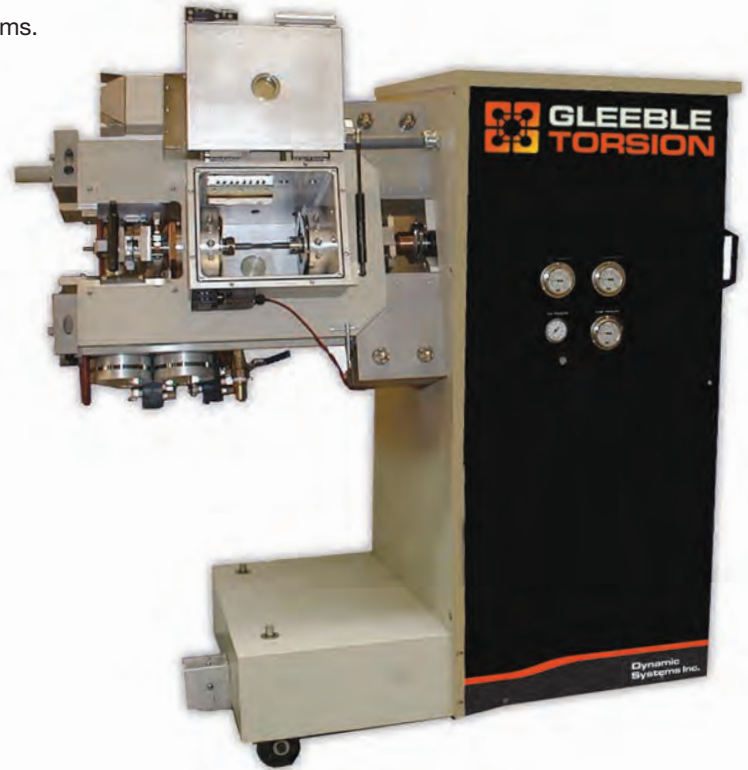
The Hot Torsion MCU uses a roll-on/roll-off design which allows the base Gleeble 3500-GTC and 3800-GTC to be easily converted to a hot torsion testing configuration.
