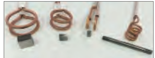
Various coil geometries are available to facilitate different types of Gleeble testing. Additional anvil materials are available.
