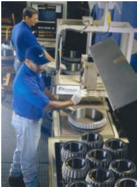
The Timken Company makes precision components, including its world famous tapered roller bearings.
