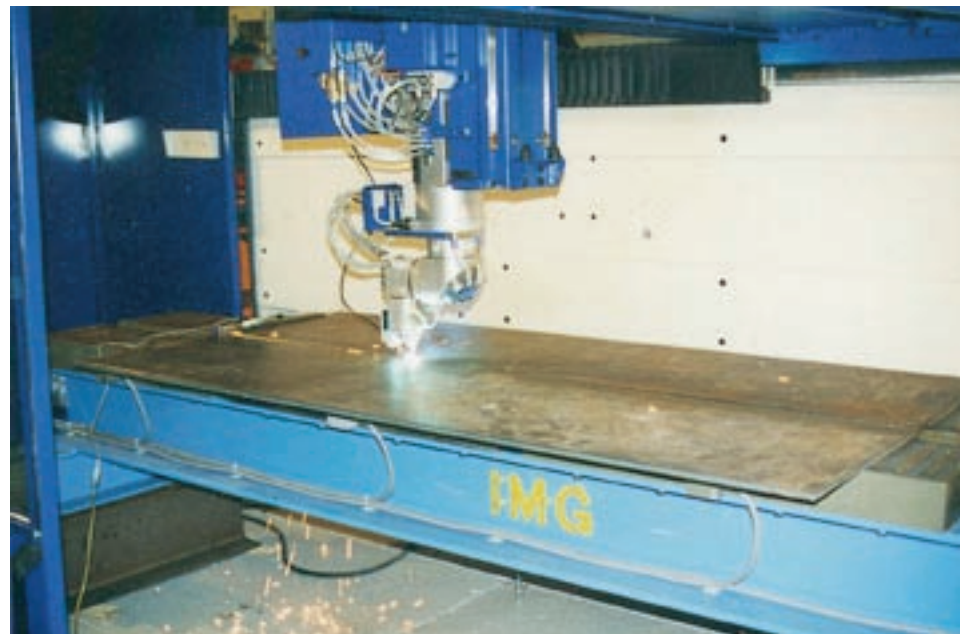
SLV's laser equipment includes a high-power CO 2 laser (12 kW output power) integrated in a six-axis beam guiding system (4 meters × 1 meter × 0.5 meter). It is able to weld a plate thickness of 15 mm in one pass.
