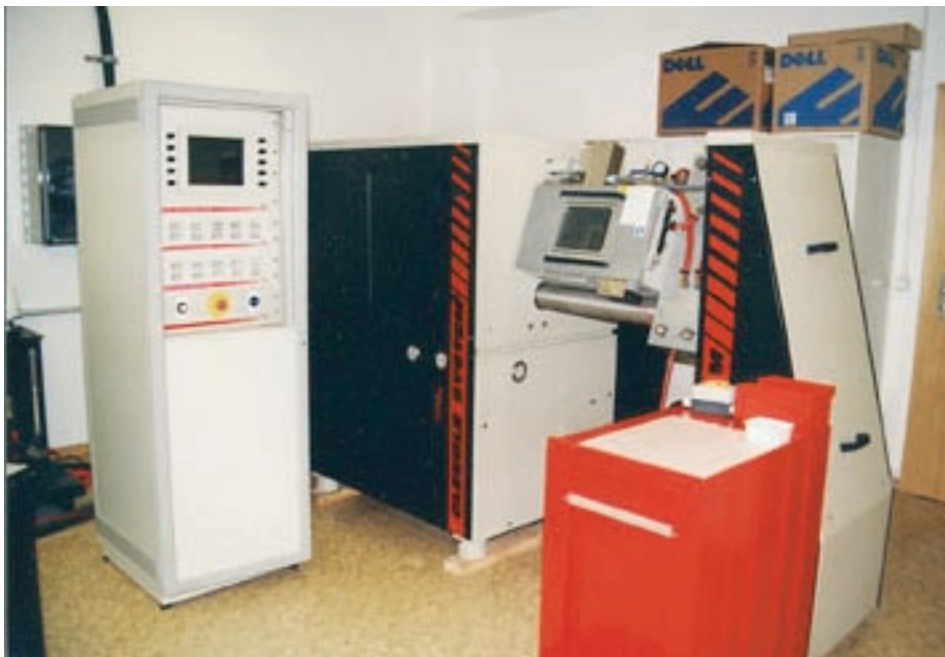
Top: This transformation diagram shows laser welding time-temperature-transformation for high strength structural steel S690Q. Bottom: SLV's Gleeble 3500 system.
