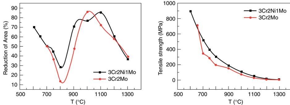
Figure 4. Typical hot tensile mechanical properties: (left) hot ductility as a function of temperature; (right) hot tensile strength as a function of temperature.
