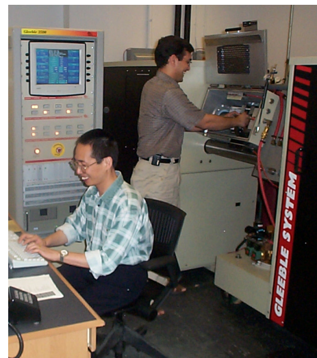
Students Gang Shi (left) and Chirag Sha perform Gleeble tests on 1080 steel, standard specimen type N, at IIT's Thermal Processing Technology Center.
