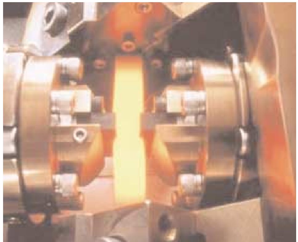
The MAXStrain multi-axis hot deformation system is capable of producing strain as high as 15 and beyond. To do so, it restrains up to a 25 mm square × 185 mm long specimen lengthwise while allowing unlimited deformation in the other two dimensions.
