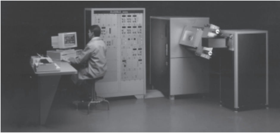
The new Gleeble 2000, Model 20:10, shown here with optional Hydrawedge, offers maximum static force capacity of 20 tons in compression and 10 tons in tension.
