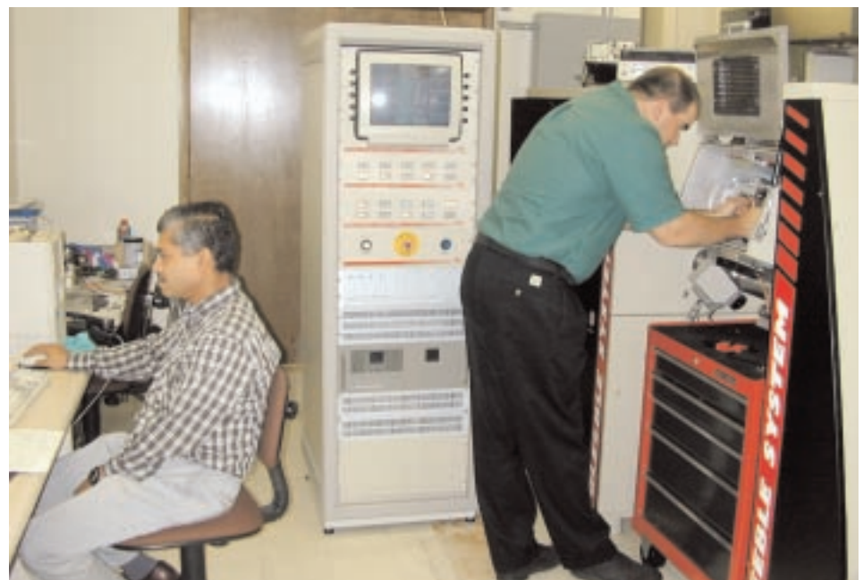
Matthew Merwin (right), Senior Research Engineer, and Kalyan Khan, Associate Research Consultant, prepare to run a simulation on U. S. Steel Group's Gleeble 3500.
