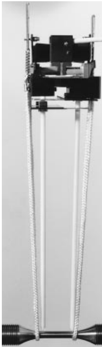
Left: Model 39016 CCT Dilatometer kit. Top: The 39070/39071/39072 Hot Zone L-Strain systems.
