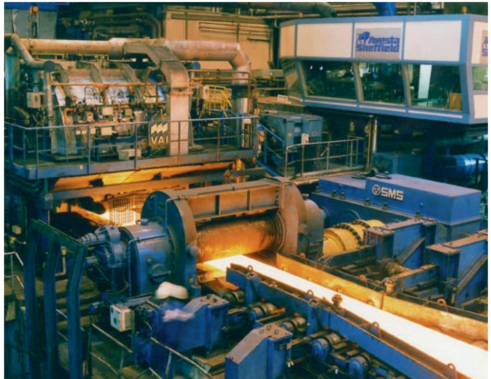
The Gleeble makes it possible to optimize the rolling sequence for special grades of stainless steel at Avesta Sheffield's Steckel mill.
