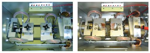
*The Gleeble is configured for nil-strength temperature (left) and with low force pocket jaws (right).*
